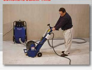
Our fleet of scarifiers is a key addition to our surface preparation arsenal as they are useful and versatile for a wide range of jobs. When used with an appropriate dust collection system, these systems control dust while scarifying, planning, cleaning and resurfacing concrete, asphalt and steel.
