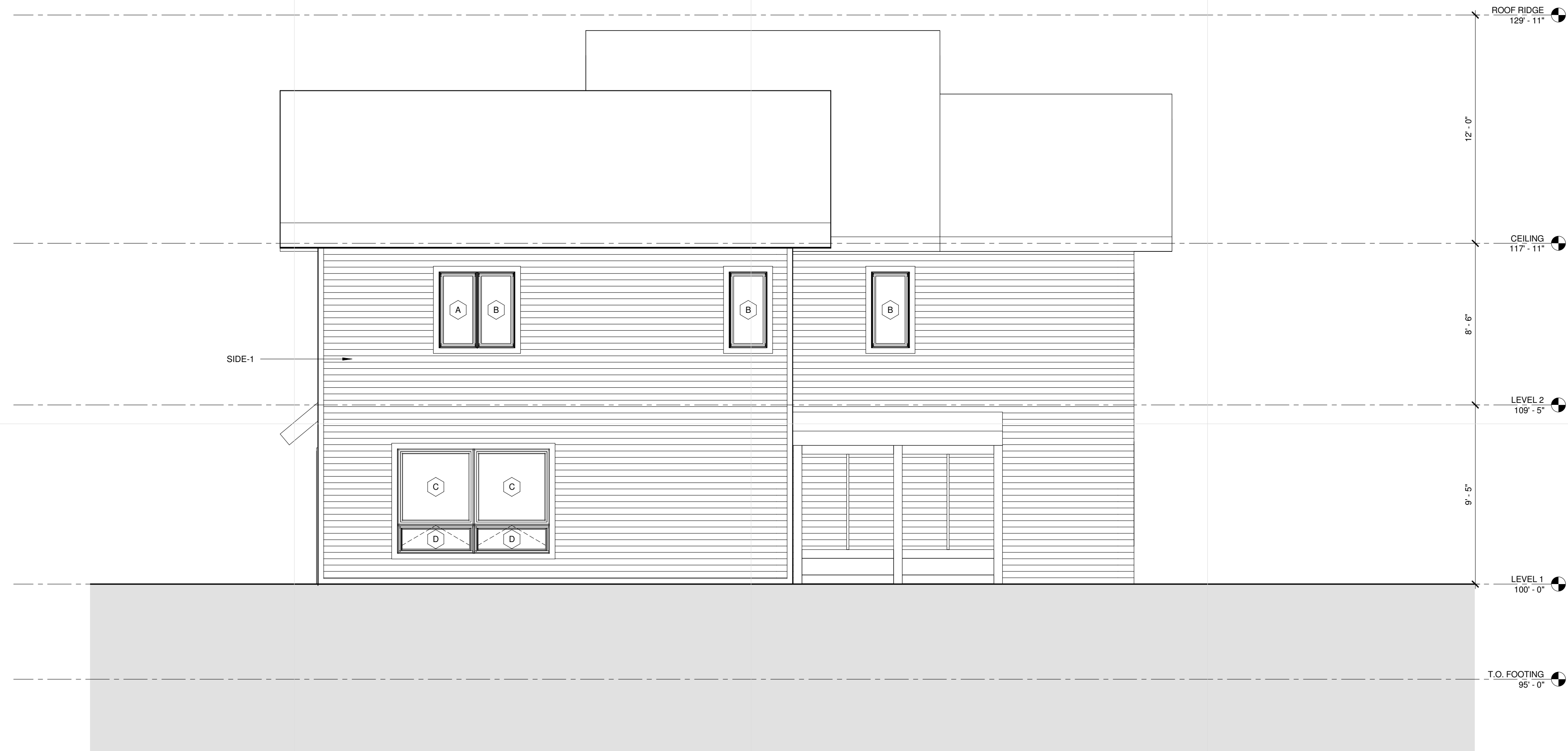
2 BUILDING NORTH ELEVATION A203 1/4" = 1'-0"
