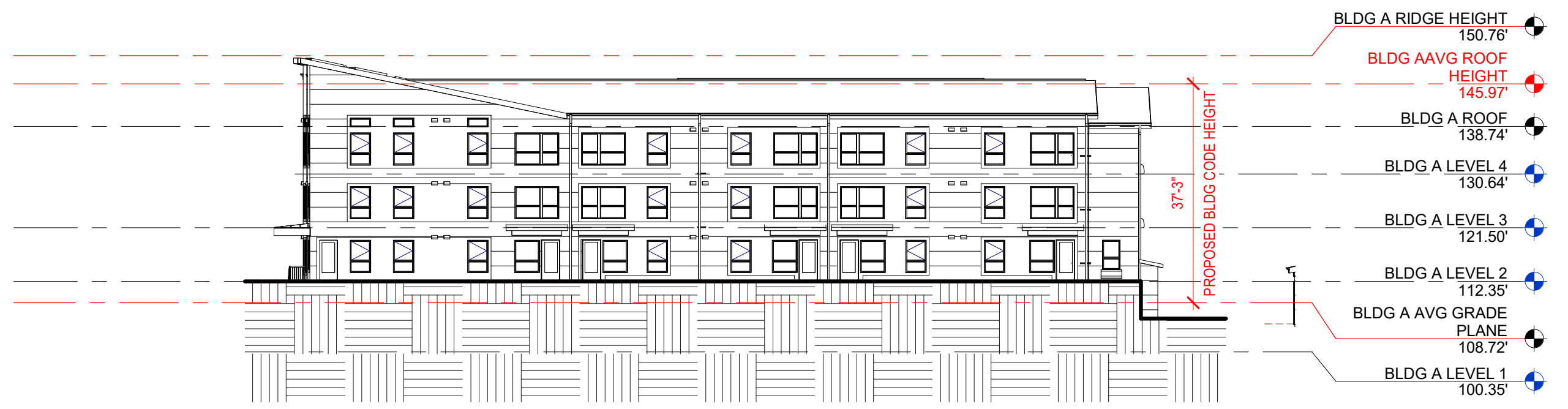
D3 BUILDING A - BUILDING CODE HEIGHT 1" = 20'-0"
