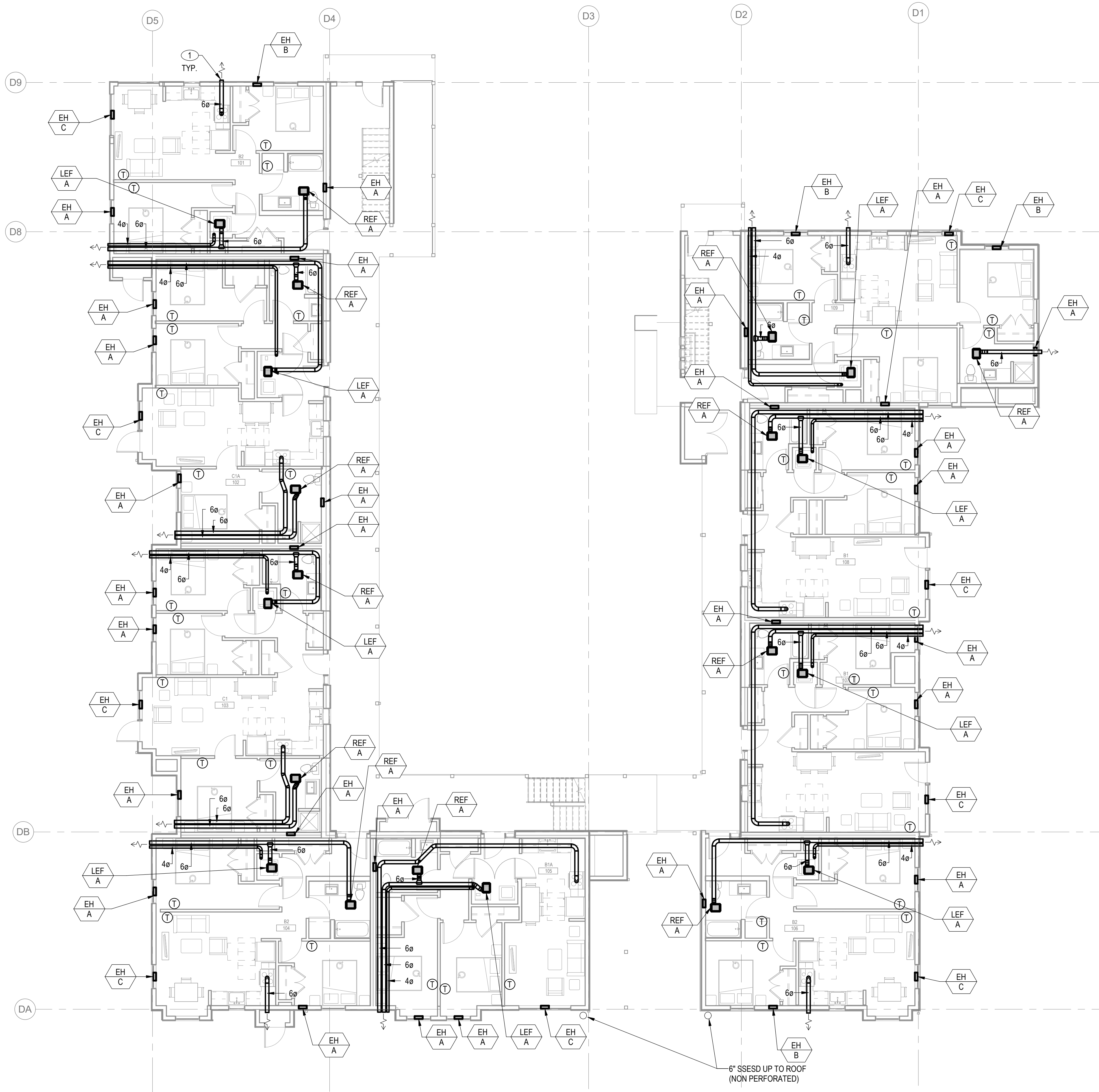
1 BUILDING D - LEVEL 1 FLOOR PLAN - HVAC SCALE: 1/8" = 1'-0"
