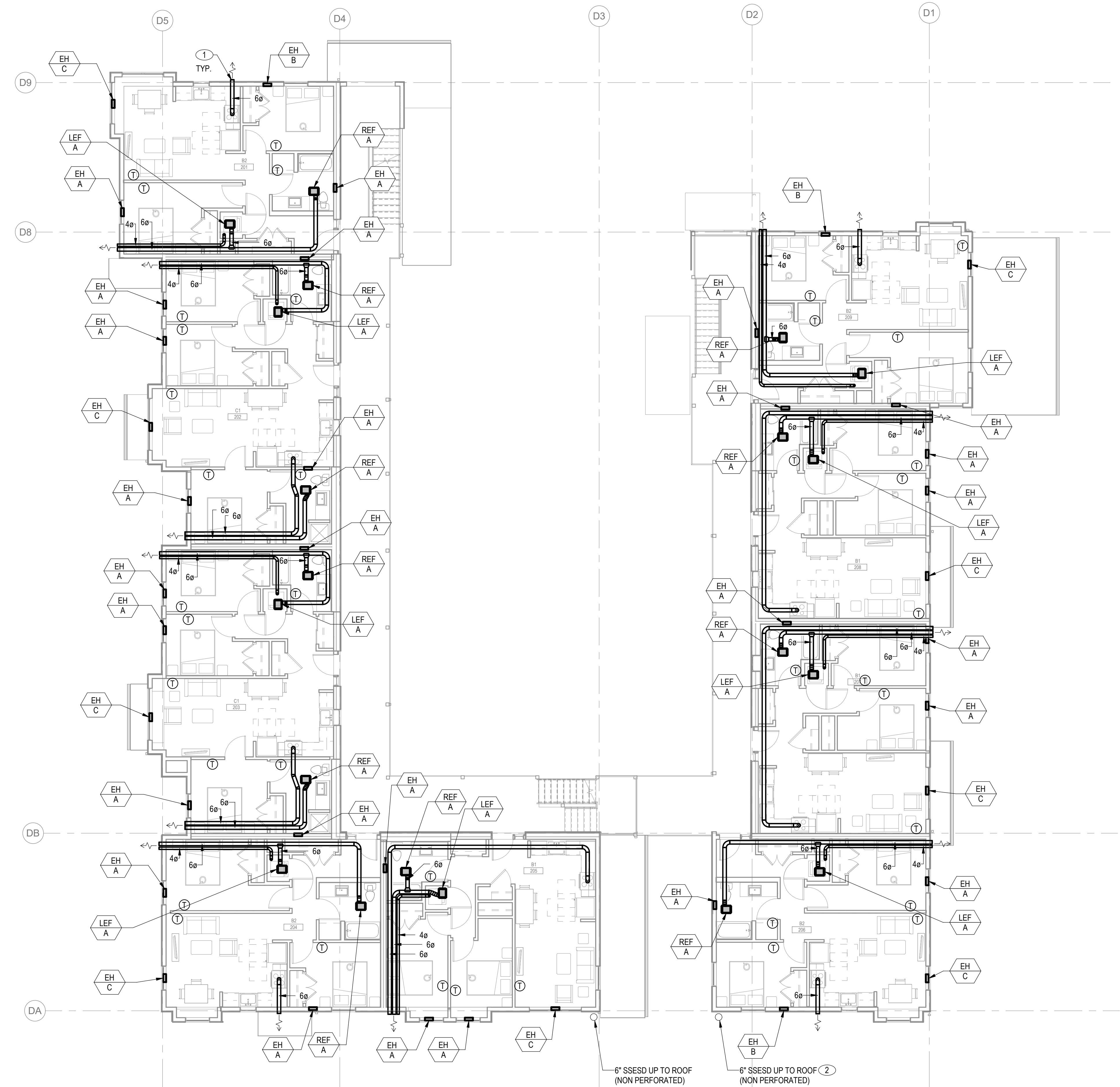
1 BUILDING D - LEVEL 2 FLOOR PLAN - HVAC SCALE: 1/8" = 1'-0"
