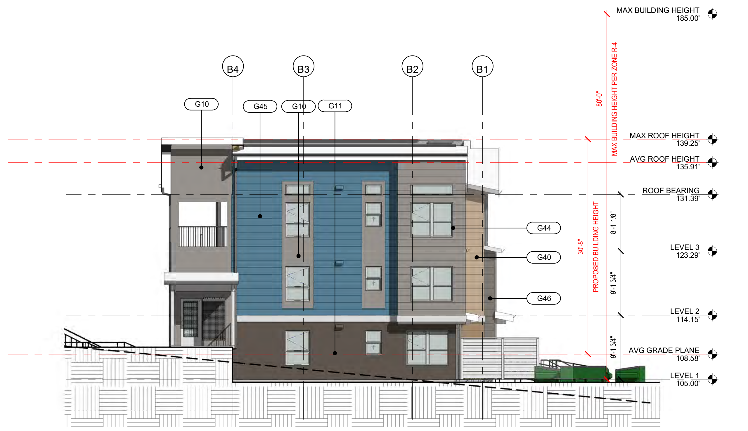
A1 BUILDING B - SOUTH ELEVATION RENDERED 1/8" = 1'-0"
