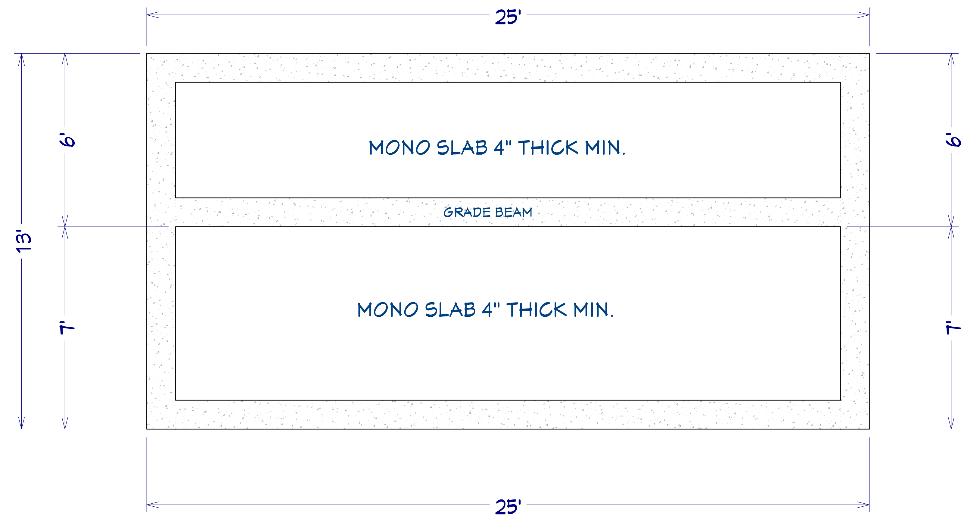
FOUNDATION LAYOUT VERIFY ALL DIMS AND PLACEMENT OF GRADE BEAMS PRIOR TO THE START OF CONSTRUCTION
