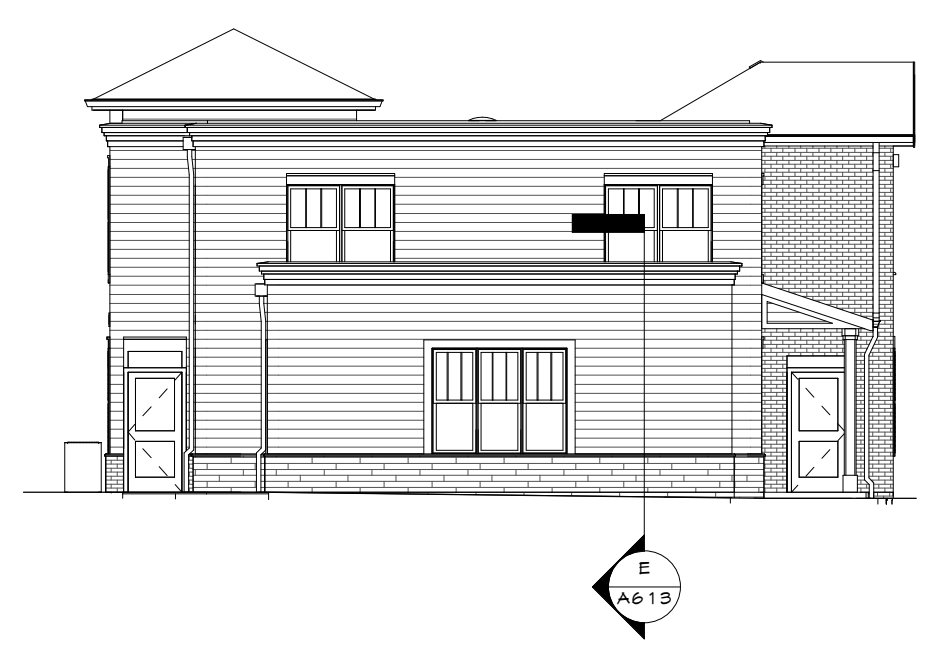
BUILDING 'D' EAST ELEVATION 3/32" = 1'-0"
