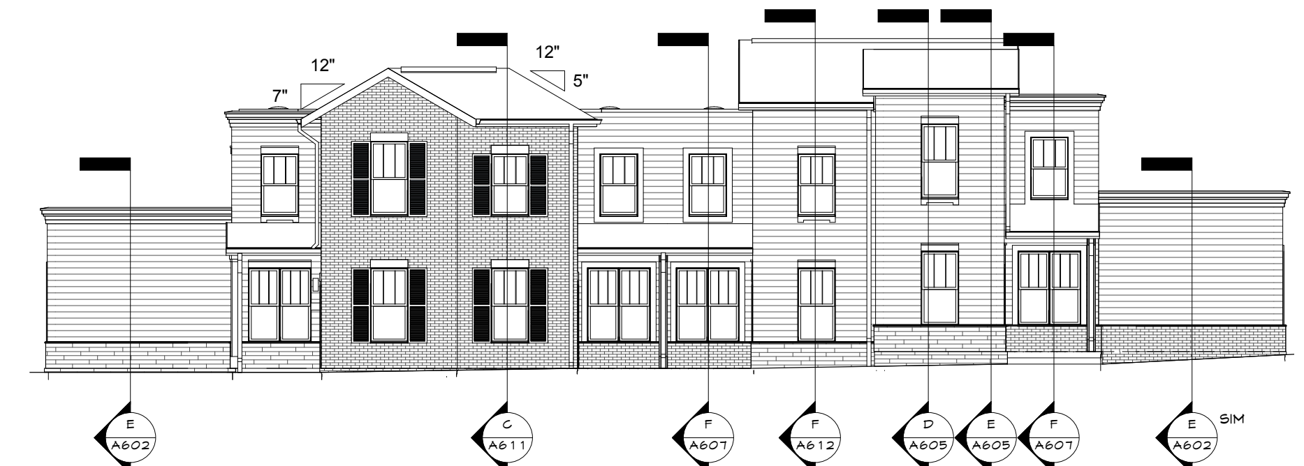
BUILDING 'D' NORTH ELEVATION 3/32" = 1'-0"
