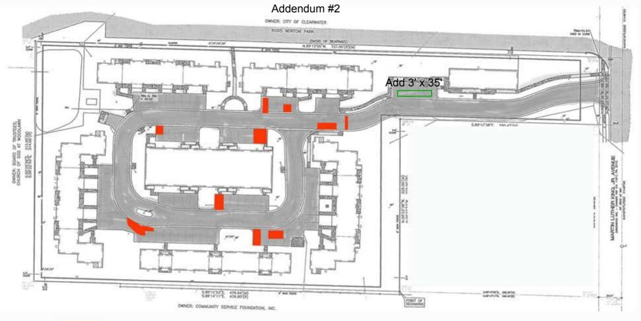
REFER TO SCOPE OF WORK TACK COAT REPAIRS. RED AREAS ARE NEAR THE FOL-LOWING LOCATIONS: PARKING SPOTS 203, 201, 701-702, 706, 506, 710, 502, 501, 601 AND (2) SPEED BUMPS. LOCATIONS ARE ALSO MARKED ONSITE.
