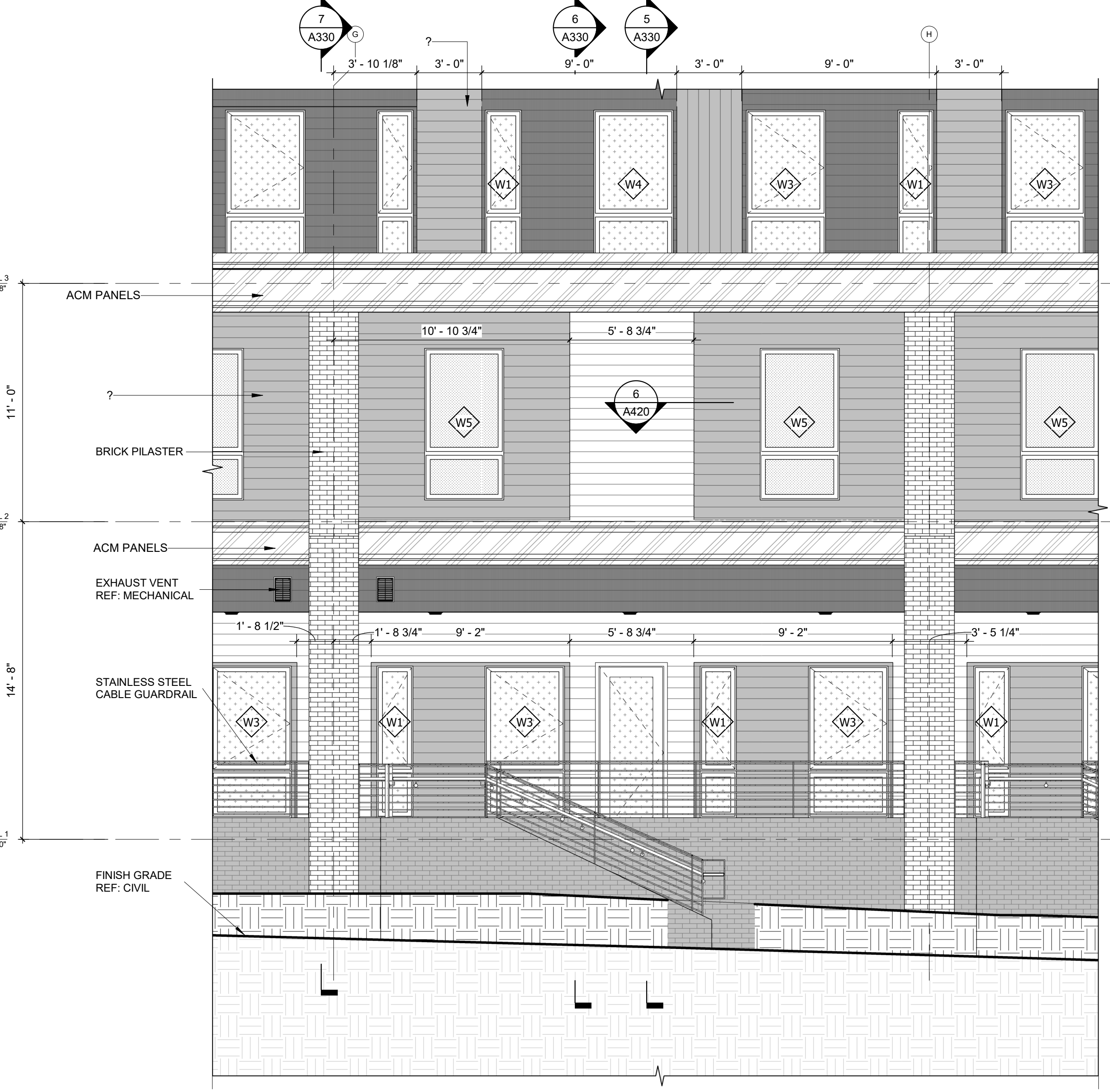
4 ENLARGED ELEVATION - S 5TH STREET 1/4" = 1'-0"
